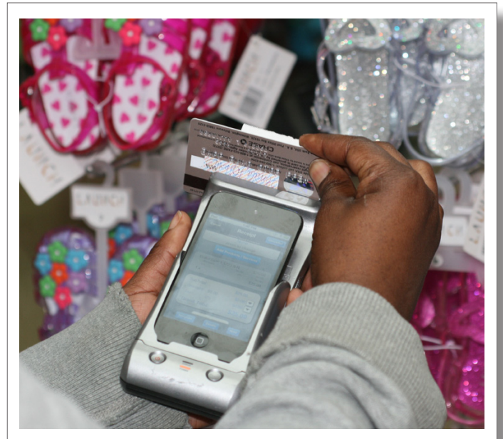
The iAPS sled adds bar code scanning, card swiping and receipt printing to the iPod touch, providing a complete mobile POS solution.
